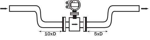
D= Diameter of Flow Meter in Inch
